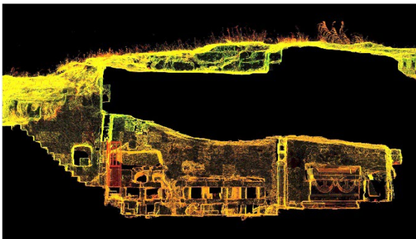
Figure 10. Roman hypogeum, shaded point cloud, long section.
