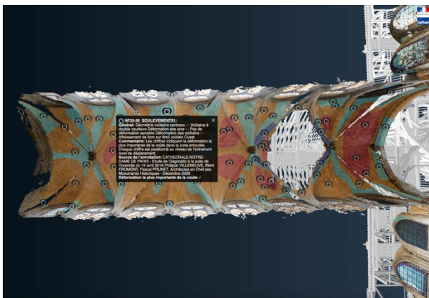
Figure 7. Visualization of a deformation layer pour the vaults of the nave, in the ND viewer
