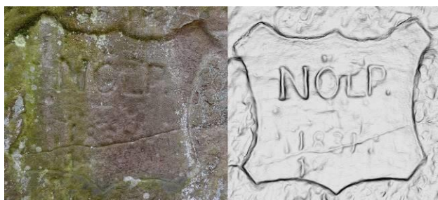
Figure 15. Comparison of almost illegible graffiti on the left (photograph) and, on the right, virtually illuminated 3D surface model.
