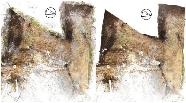
Figure 5. Overview of the quarry; point cloud from the TLS-data (left), ground floor-section of the point cloud at the level of the stone walls (right).
