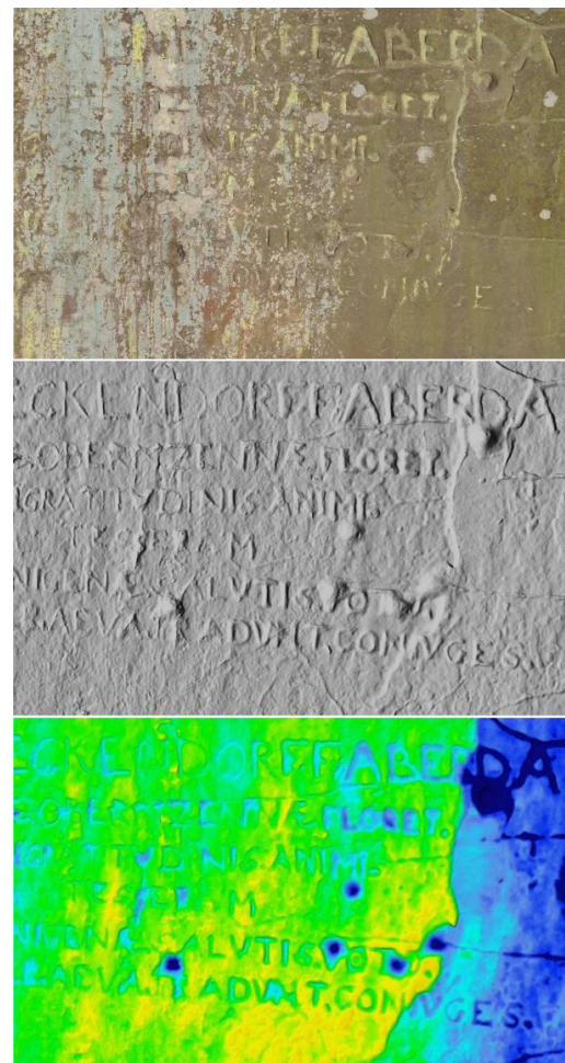
Figure 9. Detail orthophotos of the SLS-data of a memorial inscription on the western wall (wall 2) to enhance the readability of the inscriptions (from top to bottom): textured 3D model, textureless 3D model with raking light, depth map from a 3D comparison to a base-level (also usable for future monitoring).
