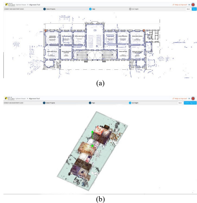
Figure 8. Point cloud alignment inside Holobuilder. Two points picking on the plan (a) and elevation definition between the point cloud and floor level (b)
