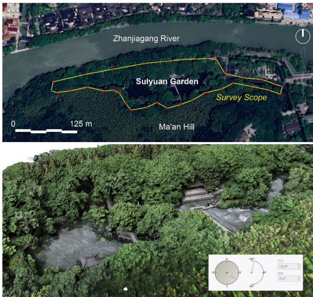
Figure 3. The survey scope and the mesh model of Suiyuan Garden created by digital photogrammetry
