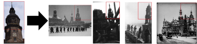
Figure 7. Left side of the arrow shows the query image depicting the top of a tower. Right of the arrow are the best results for image parts found by the neural network in the archives. The right image shows a bounding box where mainly the sky is detected.
