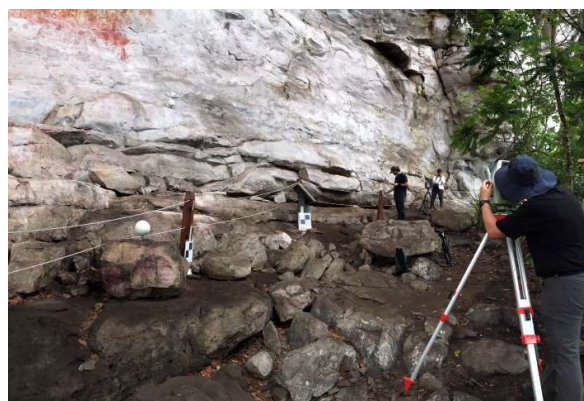
Figure 2. Acquisition of geo-referenced data with a total station.
