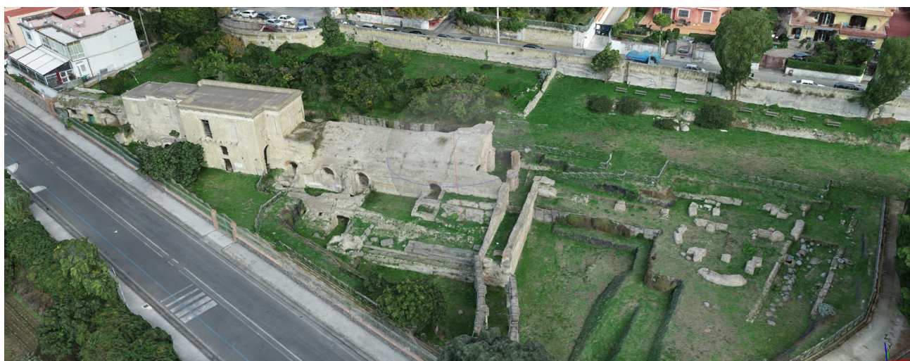
Figure 7. Perspective view of the dense point cloud from the RPAS (Remotely Pilot Aircraft System) of the Stadium of Antonino Pio.
