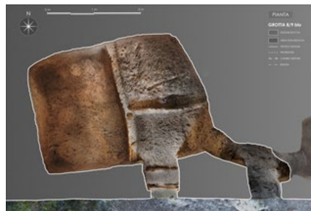
Figure 6. Covetes de los Moros. Bocairente. The 8-9 blue caves. Section and plan. Texturing in Metashape Pro.
