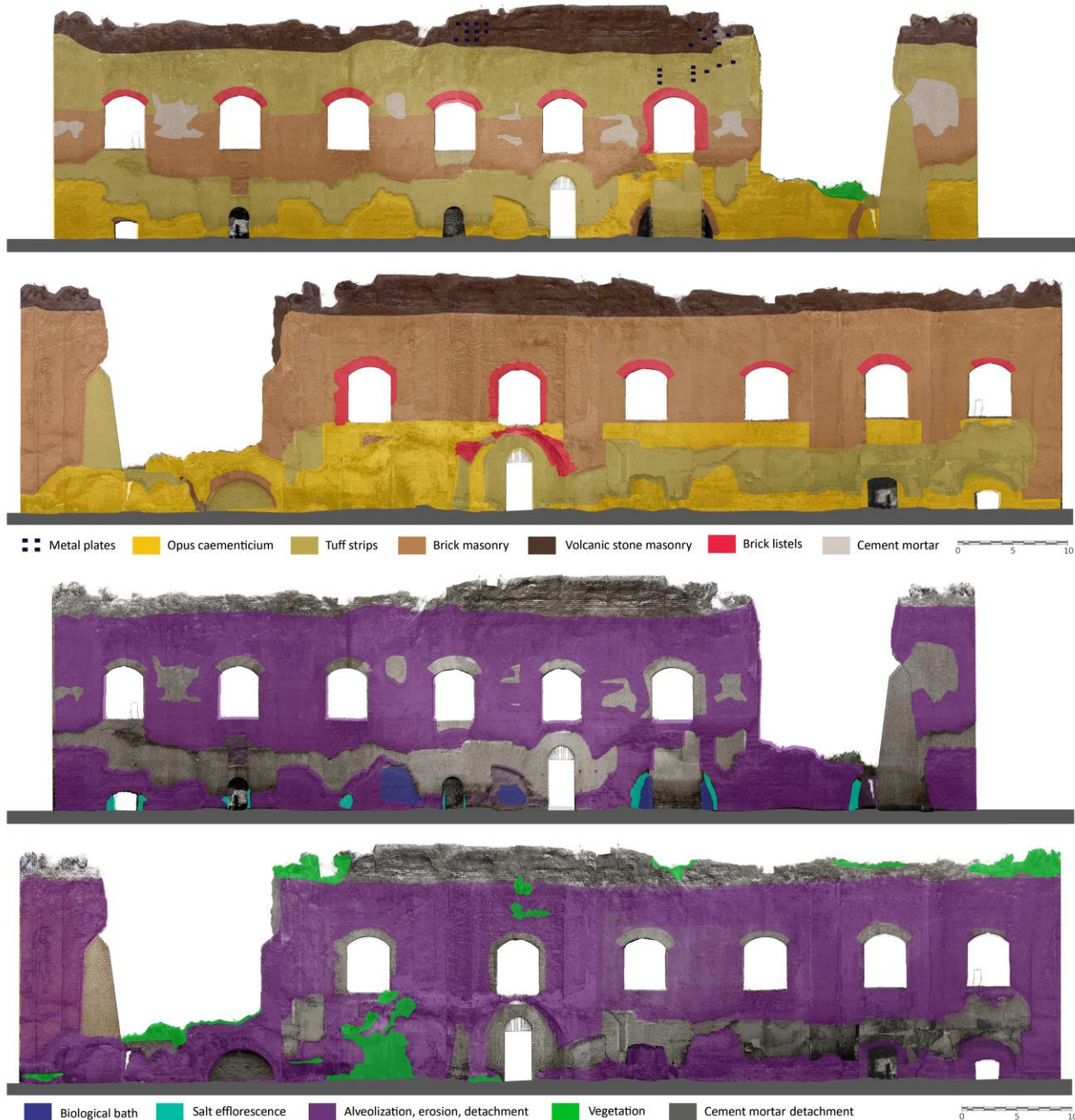
Figure 6. Result of the semi-automatic thematization of the material characterization and degradation conditions of the artefact.
