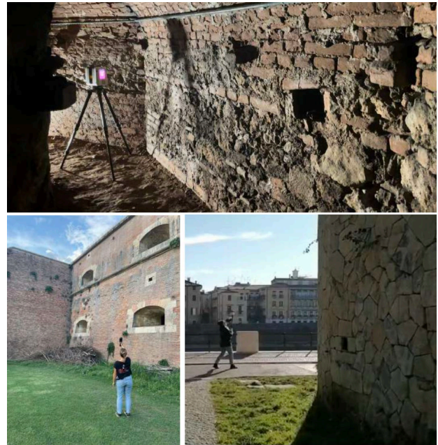
Figure 5. Laser scanner acquisition operations along the path of the magisterial walls. For the digitization of the walls, static laser scanning technologies were used, integrated through rapid mobile acquisition procedures.
