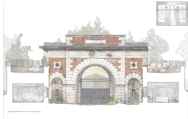
Figure 8. Section of Campofiore Gate, processed from the 3D point cloud survey data.
