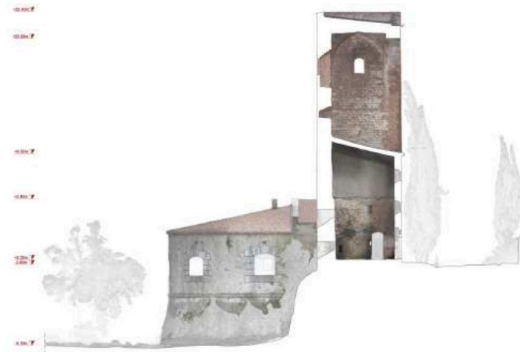
Figure 9. Section of the Scarpa battery tower, processed from the 3D point cloud survey data.
