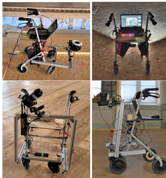
Figure 6. CHAPI in use in Ansbach (top), and Rheinsberg (bottom). Note the added weight bags in the Ansbach configuration, needed to balance the weight of the ringflash. Light (for navigation) was provided by an LED lamp.
