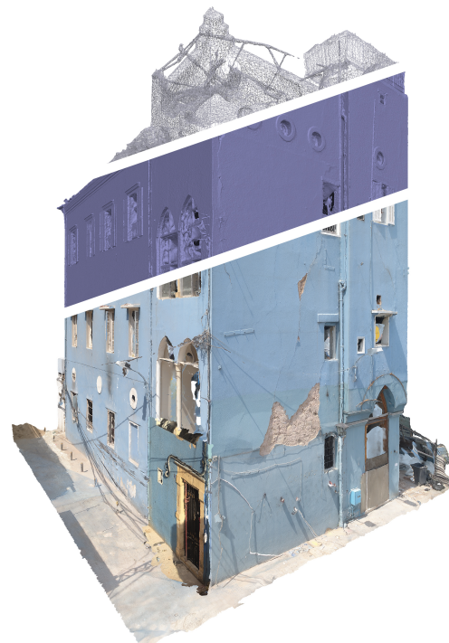
Figure 1. 3D photogrammetric model conducted by the author of one of the damaged historic buildings in Beirut following the explosion of August 4th, 2020.
