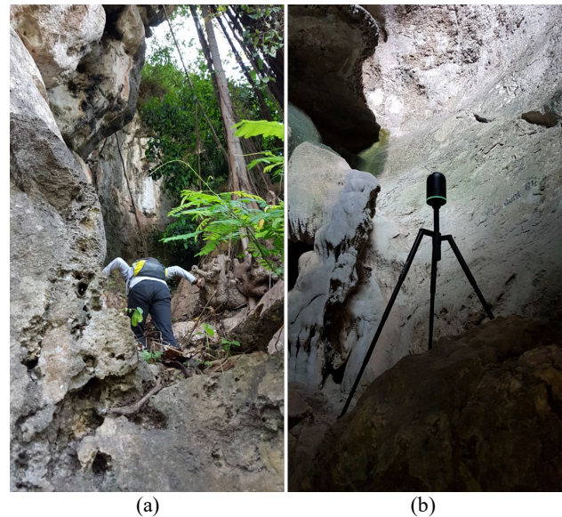
Figure 4. Terrain condition to the entrance of Barong cave. (a) Illustration of the terrain condition leading to the entrance of Barong cave. (b) Lightweight terrestrial laser scanner suitable for backpack use, used for the scanning process.
