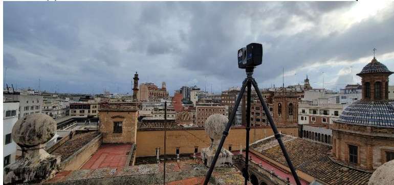
(b) A FARO Focus S-350 Laser Scanner scans the roof.
