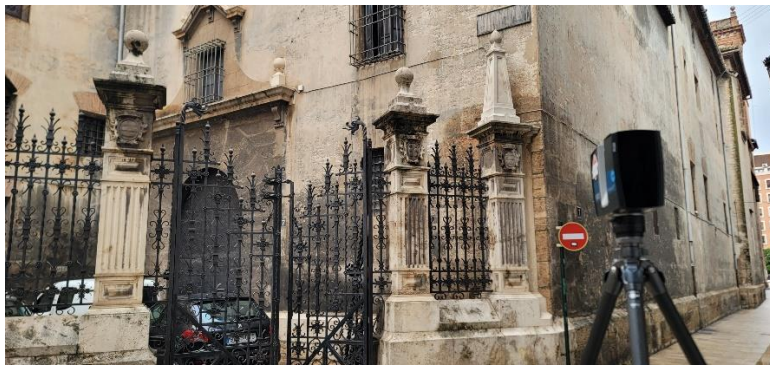
(a) A FARO Focus S-350 Laser Scanner scans the exterior façade.
