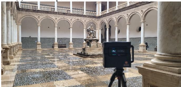
(b) A Matterport Pro2 camera scans the cloister.
