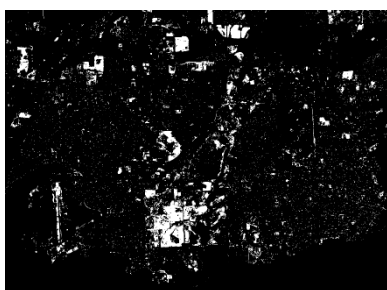
Figure 6. Change map created using MLPNN classifier and image differencing.
