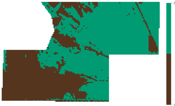
Figure 9. Binary Map generated using AP. Cluster averages using AP were calculated, and their overall average was used as a cutoff to divide clusters into high (green) and low (brown) classes.
