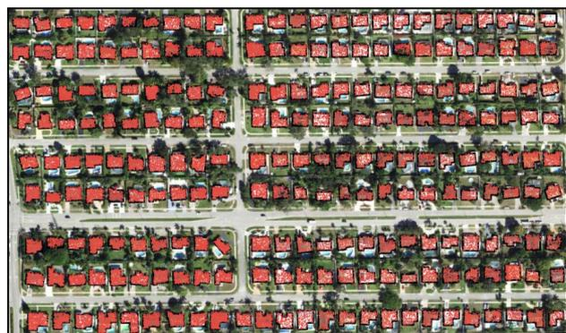
Figure 12. The improvised building points classification overlaid with the building footprint vector layer.
