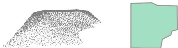
Figure 6. Side view of the point cloud of a single segment and vector layer generated after the simplification process.
