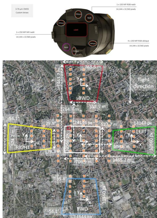
Figure 1. The ULTRACAM DRAGON 4.1 hybrid system (above). The image orientation and footprint distances in case of a flying height of approx. 1000 m (below).
