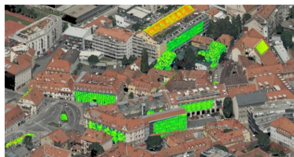
Figure 8. Examples of patches (colored regions) identified to compute the point cloud density.
