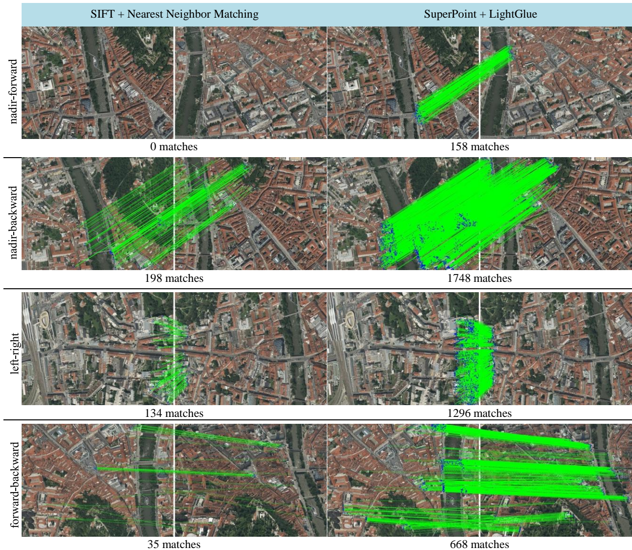
Figure 6. Matching results with a hand-crafted (SIFT) and a learning-based (SuperPoint + LightGlue) methods. Keypoints are extracted and matched at full image size (14144 x 10560 px) using the DIM tiling strategy.
