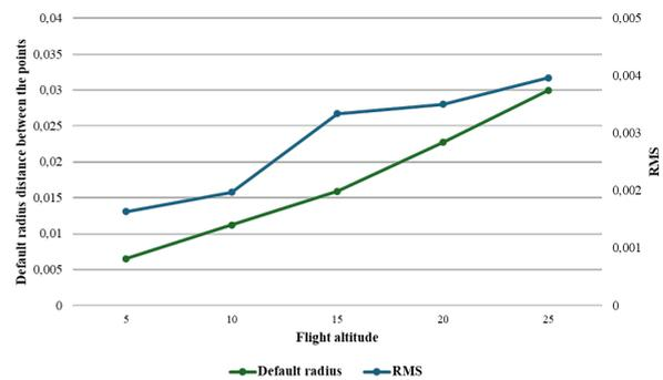
Figure 9. Default radius values calculated by CloudCompare as survey altitude increases.
