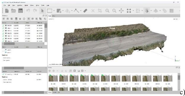
Figure 4. Dense point cloud reconstruction in Agisoft Metashape® software.
