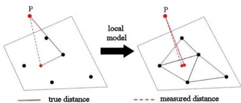
Figure 6. Schematic representation of the local 2D1/2 Triangulation model.
