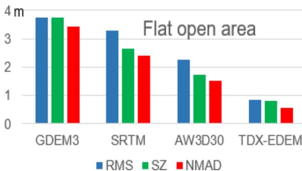
Figure 10. Accuracy of DEMs in open area of test site Flat.
