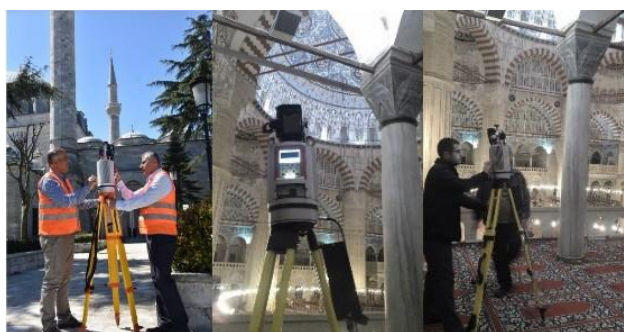
Figure 3. Terrestrial laser scanning (TLS) of the Selimiye Mosque using the integrated DLSR camera Nikon D700 on top.
