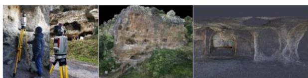
Figure 9. Terrestrial laser scanning using the Riegl VZ-400 inside and outside the cave (left) and the coloured point cloud data outside (left) and inside the cave (right).
