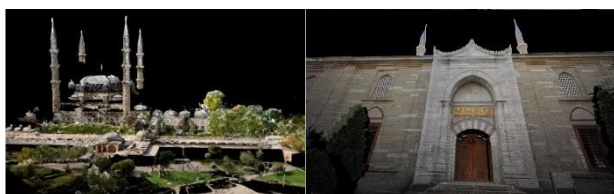
Figure 4. Part of the coloured TLS point cloud of the Edirne mosque – overview (left) and detail (right).
