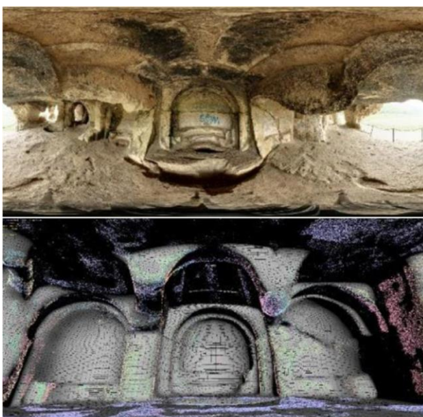
Figure 10. Gigapixel panorama of the cave indoor (top) and 3D interior model generated from the point cloud in 3ds max (bottom).
