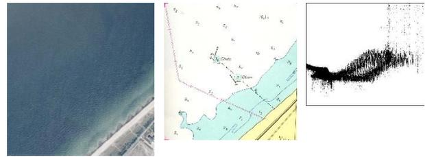
Figure 20. Relationship of water depth and grey values. Left: 6.35 m depth Right: 0.0 m.
