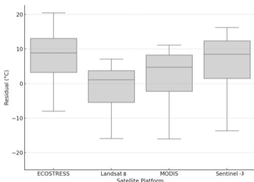
Figure 3. Distribution of residuals ( $T_{sat} - T_{ground}$ ) for each satellite platform.
