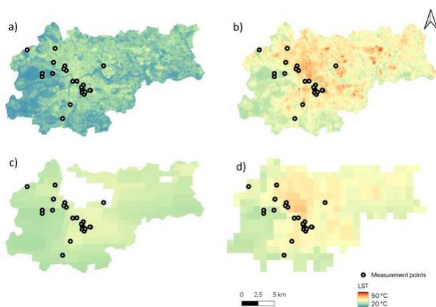
Figure 2. Land surface temperature (LST) retrieved from each satellite platform. a) Landsat 8 (100 m), b) ECOSTRESS (70 m), c) MODIS Terra (1 km), d) Sentinel-3 (1 km). Black dots indicate in-situ sensor locations (n = 27).
