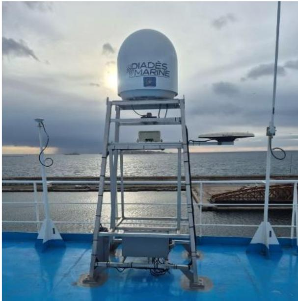
Figure 8. The sensors are located on a dedicated mast fabricated for the project and installed at the front of the ship: The radar dome on the top, the 3D LiDAR below and underneath it the cameras. A GPS antenna is installed on the right side of the mast.
