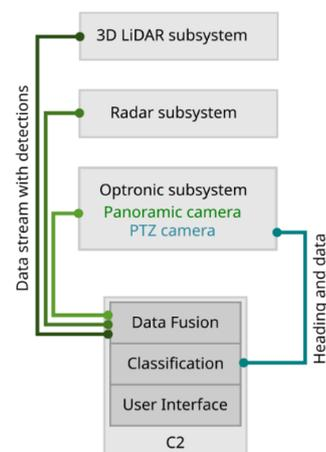
Figure 7. Overall system architecture of the OCDS.
