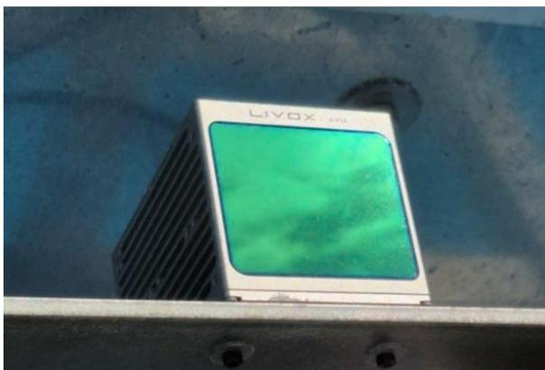
Figure 10. The Livox Avia 3D LiDAR scanner.
