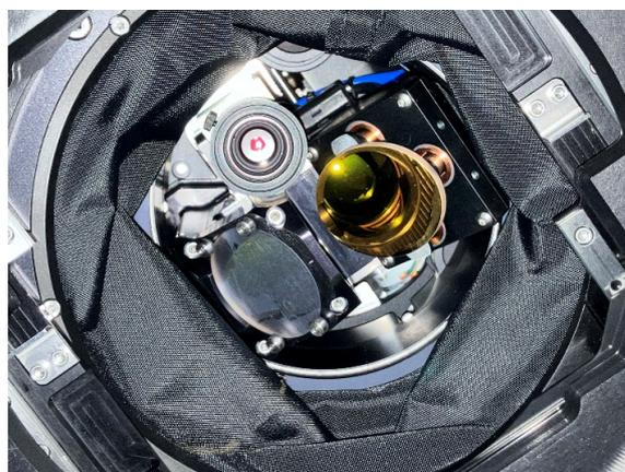
Figure 3. Hyperspectral FTIR sensor in combination with integrated RGB viewfinder camera.
