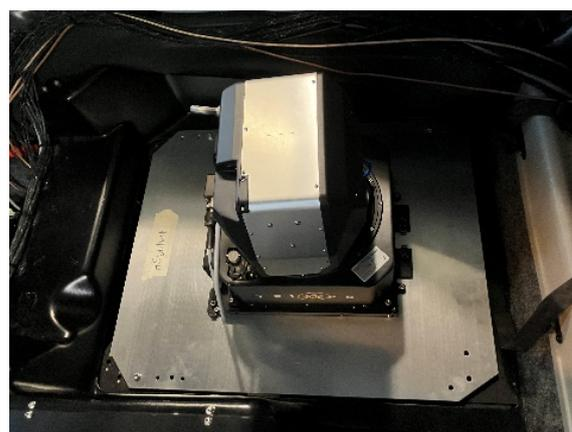
Figure 2. DA-62 adapter plate mounted into aircraft
