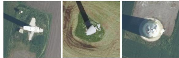
(a) Example detections of the YOLO model showing three different wind turbines. These detections were cut out and used for training the classification CNN.
