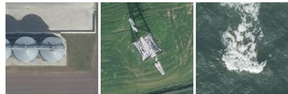
(b) Negative detections of the YOLO model that show no relevant objects for the classification. You can see a silo in the first image, a power pole in the second image and a wave in the third image.
