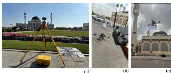
Figure 5. Site documentation process (a) Setting up GSD points, (b) Defining flight path, (c) Flying on defined flight path.
