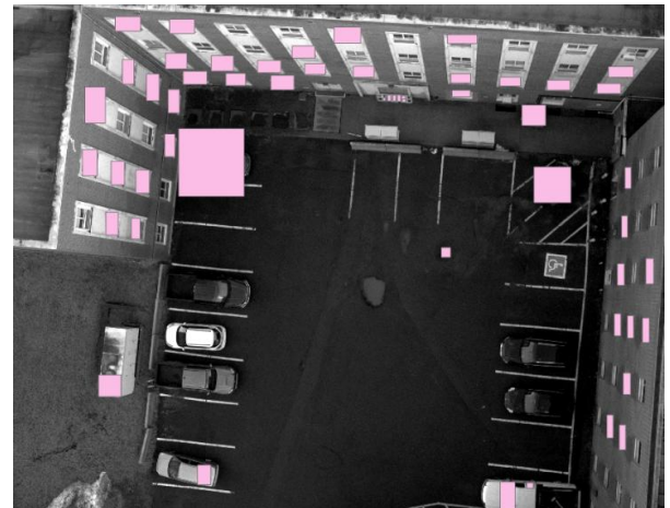
Figure 2. Example Output of 2D Imagery-Based Window Detection Using Deep Learning
