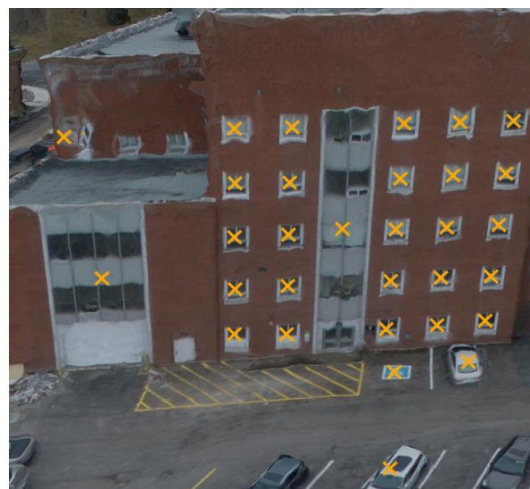
Figure 5. 3D Mesh-Based Window Detection Using Esri's Pretrained Deep Learning Model
