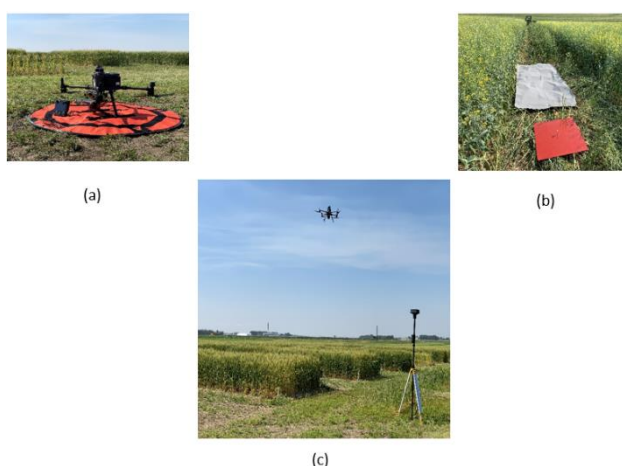
Figure 3. Photos of some steps of data collection conducted in this project. (a) UAV equipped with MSI sensor before flight, (b) calibration tarp used for radiometric calibration of taken images, (c) UAV over the crops with GPS instrument to orthorectify images.
