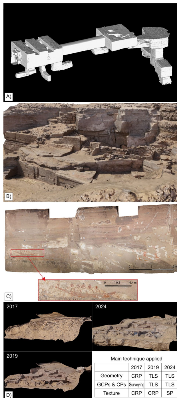
Figure 6. Examples of the results obtained: a) 3D mesh of QH36; b) 3D model of the exterior area next to QH34cc; c) orthoimage of the northern wall of the hall of pillars (QH36); d) evolution of the documentation carried out in different campaigns (exterior area next to QH34).
