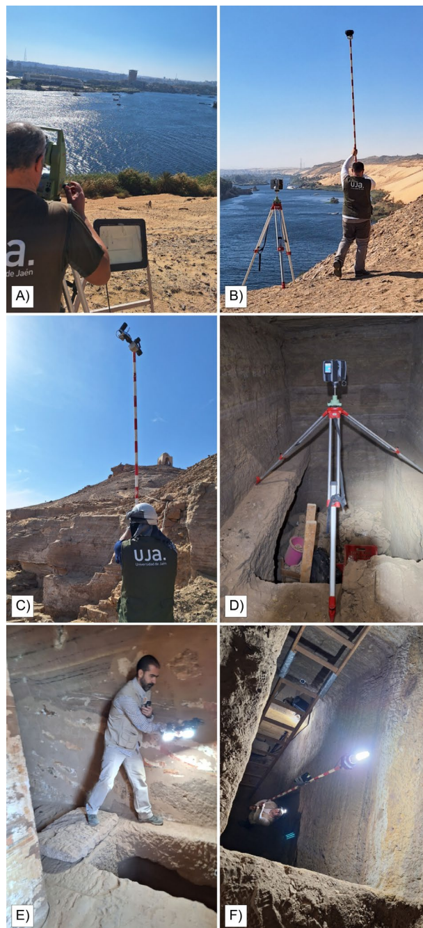
Figure 3. Images of the application: a) Surveying network (exterior); b) TLS and SP (exterior); c) CRP from a mast (exterior); d) TLS (interior QH36); e) CRP (interior QH36); f) SP from a mast (interior QH36).
