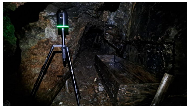
Figure 5. Measurement with TLS Leica BLK360
