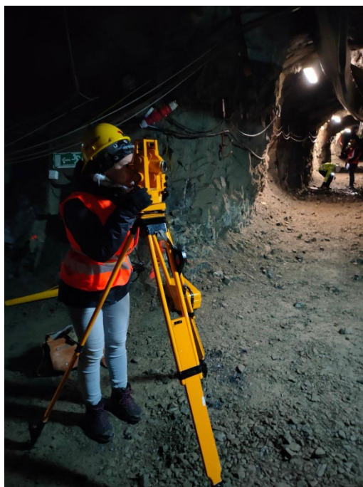
Figure 4.: Positioning the point field using the theodolite
