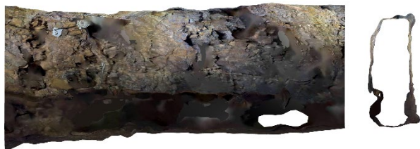
Figure 12. Textured 3D mesh of the 'U Pinců' adit generated from iPhone LiDAR data using Pix4D
