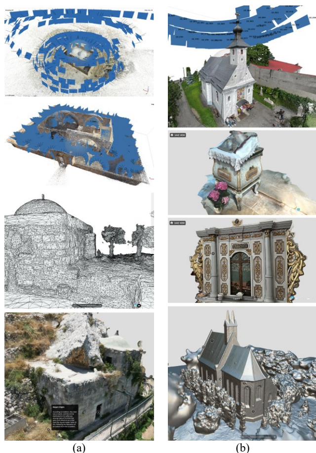
Figure 1. Examples of architectural heritage datasets used in the two workshops: (a) multi-scale documentation and 3D reconstruction of a historic Maqam (shrine) site from the Sharjah workshop (UAE); (b) photogrammetric models of churches and interior architectural elements from the Cluj-Napoca workshop (Romania).
