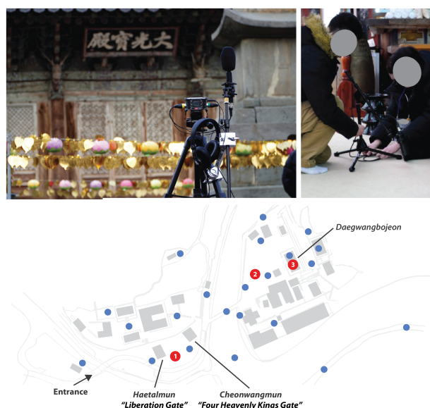
Figure 2. Top: images of outdoor and indoor ambisonic microphone recording setup at Magoksa Temple. Bottom: a map of Magoksa Temple Complex with 22 recording locations (blue), and 3 reconstructed zones (red).
