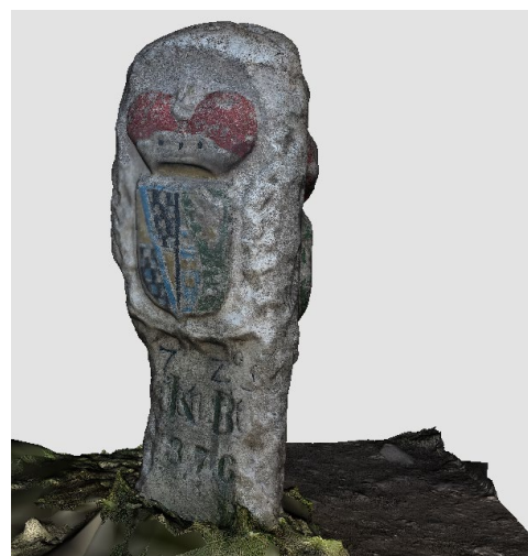
Figure 15: RCM generated mesh model, 600 thousand triangles, supported with LiDAR device, optimized fully automatically taken photos
