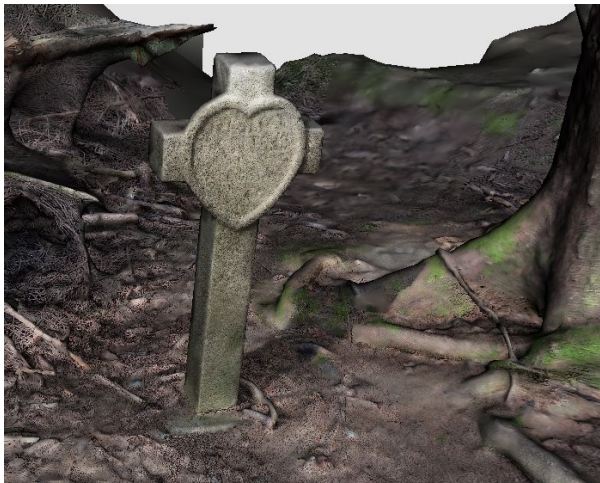
Figure 11: RCM generated mesh, 600 thousand triangles
