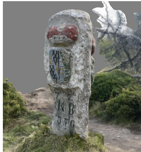
Figure 13: Agisoft Metashape generated mesh model, 118 photos, hand-held taken photos
