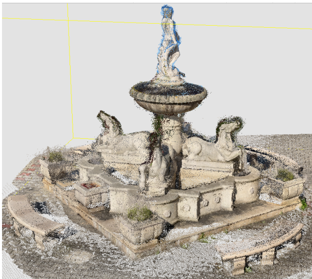
Figure 6: point cloud derived from videogrammetry, 3DSurvey, 2.3 million points, 616 photos generated from video
