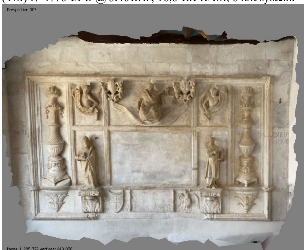
Figure 17: Agisoft Metashepe, 20 photos, 2 minutes capturing, 15 minutes of processing on workstation, meshed and textured 3D model 1.2 million triangles, 10.6 million points
