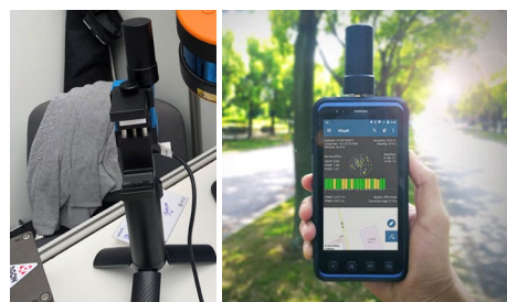
Figure 2. Smartphone with connected RTK GNSS, 3DSurvey
