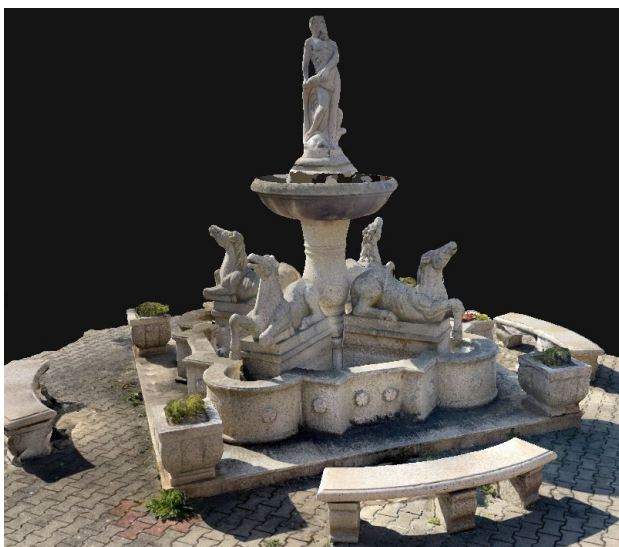
Figure 7: point cloud from ViDoc reduced on 5 million points, 27 million points originally
