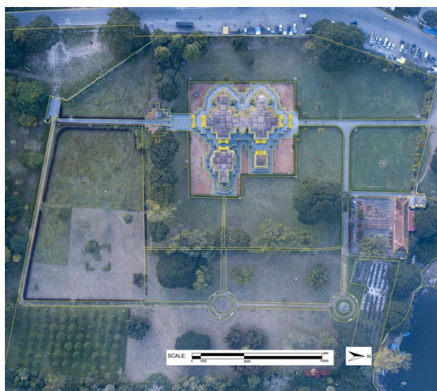
Figure 2: Site plan of the Halebidu Temple, produced through drone photogrammetry. Reference scale included.
