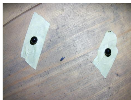
Figure 2: Two black spheres under the dome for the calibration measurement (Richter 2025).
