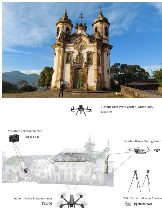
Figure 5. Application of equipment for reality capture according to their respective technology.
