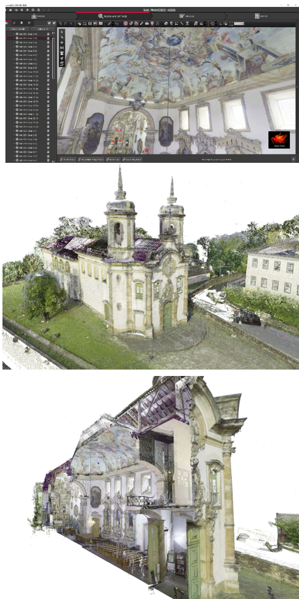
Figure 7. Sample of point cloud captured by laser scanning with millimetric precision.
