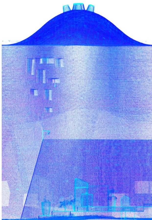
Figure 8. Vertical section of the point cloud highlighting the gaussian vault conceived by Dieste. The final high density dataset obtained by the integration of heterogeneous 3D acquisition tools could enhance the knowledge on these peculiar structures.
