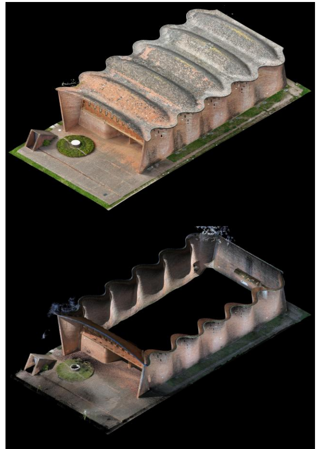
Figure 6. RGB data comparison between Leica BLK (top) and Lixel K1 equipment (down).
