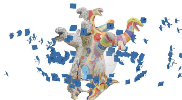
Figure 5. Camera positioning around a sculpture using combined terrestrial and aerial photogrammetry.
