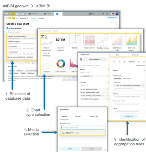
Figure 8. BI querying process scheme: from data selection to the definition of analysis metrics and aggregation rules, to generate new information viewable through dashboards.
