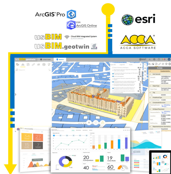
Figure 6. Preliminary results of data integration in the usBIM.geotwin platform, involving the integration of data managed in collaboration with the Esri GIS platform and through an organized collection of information via usBIM.
