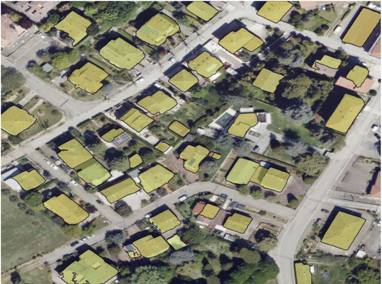
Figure 4. Refined SAM segmentation used for comparison, with internal holes removed and small segments filtered out.
