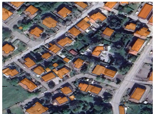
Figure 6. Comparison between satellite imagery and cadastral footprints, illustrating alignment issues due to perspective distortion in off-nadir satellite acquisition
