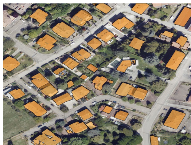
Figure 3. Initial SAM segmentation output overlaid on the orthophoto. The masks still contain internal holes and unfiltered small segments.
