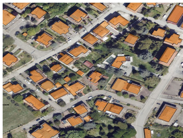
Figure 2. Overlay of the high-resolution orthophoto with official cadastral building footprints (in orange), used to assess spatial correspondence and identify discrepancies.
