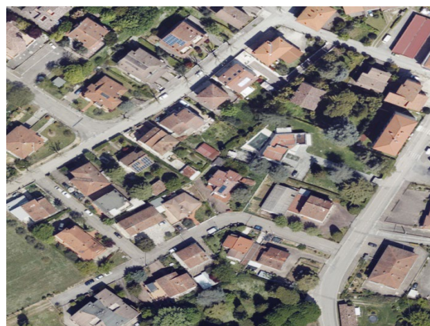
Figure 1. High-resolution orthophoto (20 cm/pixel) used as the base layer for automatic building segmentation and comparison with cadastral data.
