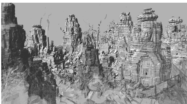
Figure 3. Point cloud data of the central temple acquired using fixed terrestrial laser scanners
