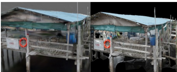
Figure 12. Side-by-side comparison of gaussian splat (left) and photogrammetry model (right)
