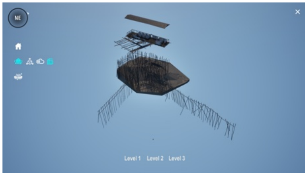
Figure 19. HBIM mode showcasing an exploded view of the different 'levels' and structural components of the kelong
