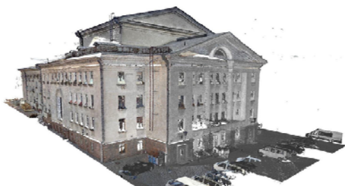
Figure 4. Overview of the combined point clouds produced by the laser scanning process. (©UNESCO/ICOMOS)
