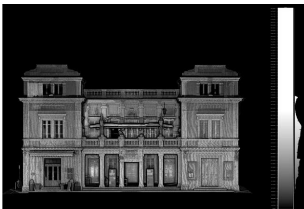
Figure 7. View of the main façade of the Teatro Nuovo in Mirandola extracted from the point cloud during the data assessment phases (graphic elaboration by the authors).
