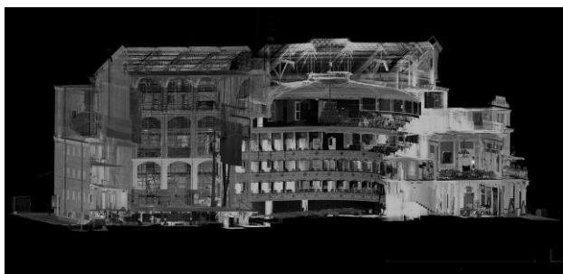
Figure 9. Axonometric section extracted from the point cloud (graphic elaboration by the authors).
