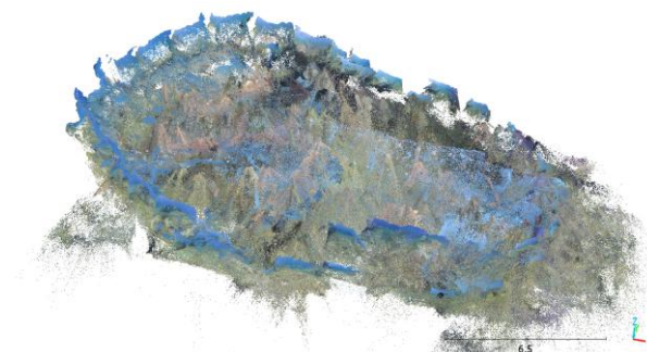
Figure 11. Point cloud generated using the Nerfacto NeRF pipeline.
