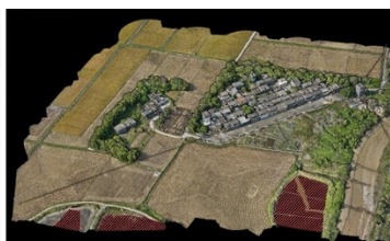
Figure 12. The final point cloud model of the case. The red shadow lines in the image below indicate missing data at the water surface
