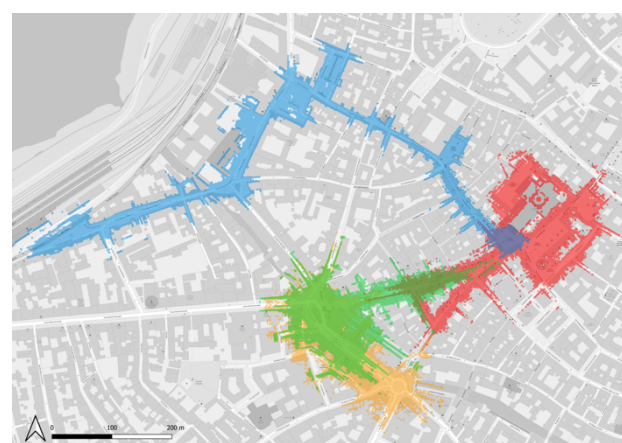
Figure 3. Map of the areas surveyed for the purposes of the project using various HMLS. In red data acquired by Stonex X120, in blue the ones acquired by Stonex X70 GO, in green the ones acquired by Emesent Hovermap, and in yellow the ones acquired by Geoslam ZEB Horizon. There is an overlapping area in the city where all instruments were used.
