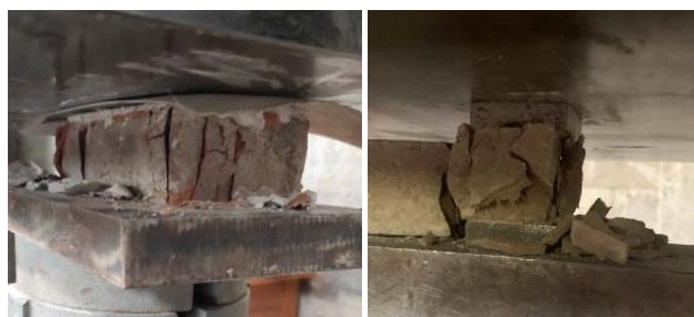
Figure 12. Compression test on a clay solid unit (left) and on a stone unit (right)
